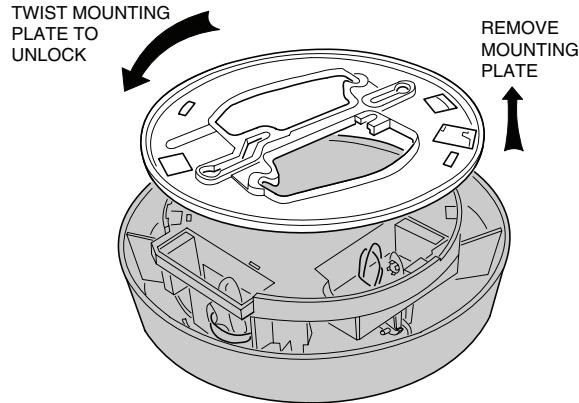
**STEP 2 Identify components.** Examine the TSD-90A to identify the component locations.
